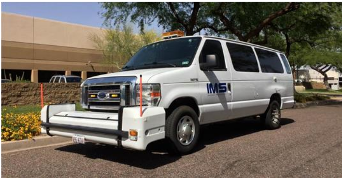
Figure 3 – Laser Road Surface Tester (RST)
