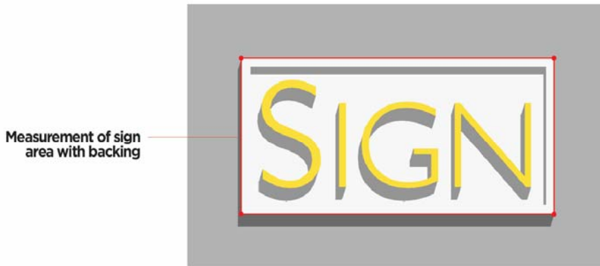
Figure 12.4(La). Sign Area for Signs with Backing
